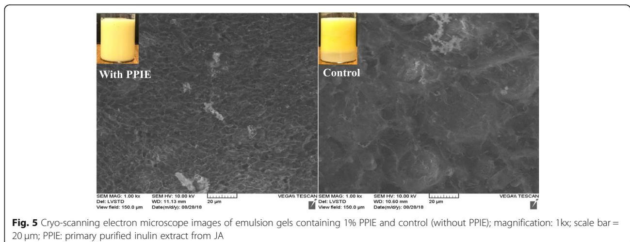
**Fig. 5** Cryo-scanning electron microscope images of emulsion gels containing 1% PPIE and control (without PPIE); magnification: 1kx; scale bar = 20  $\mu\text{m}$ ; PPIE: primary purified inulin extract from JA
