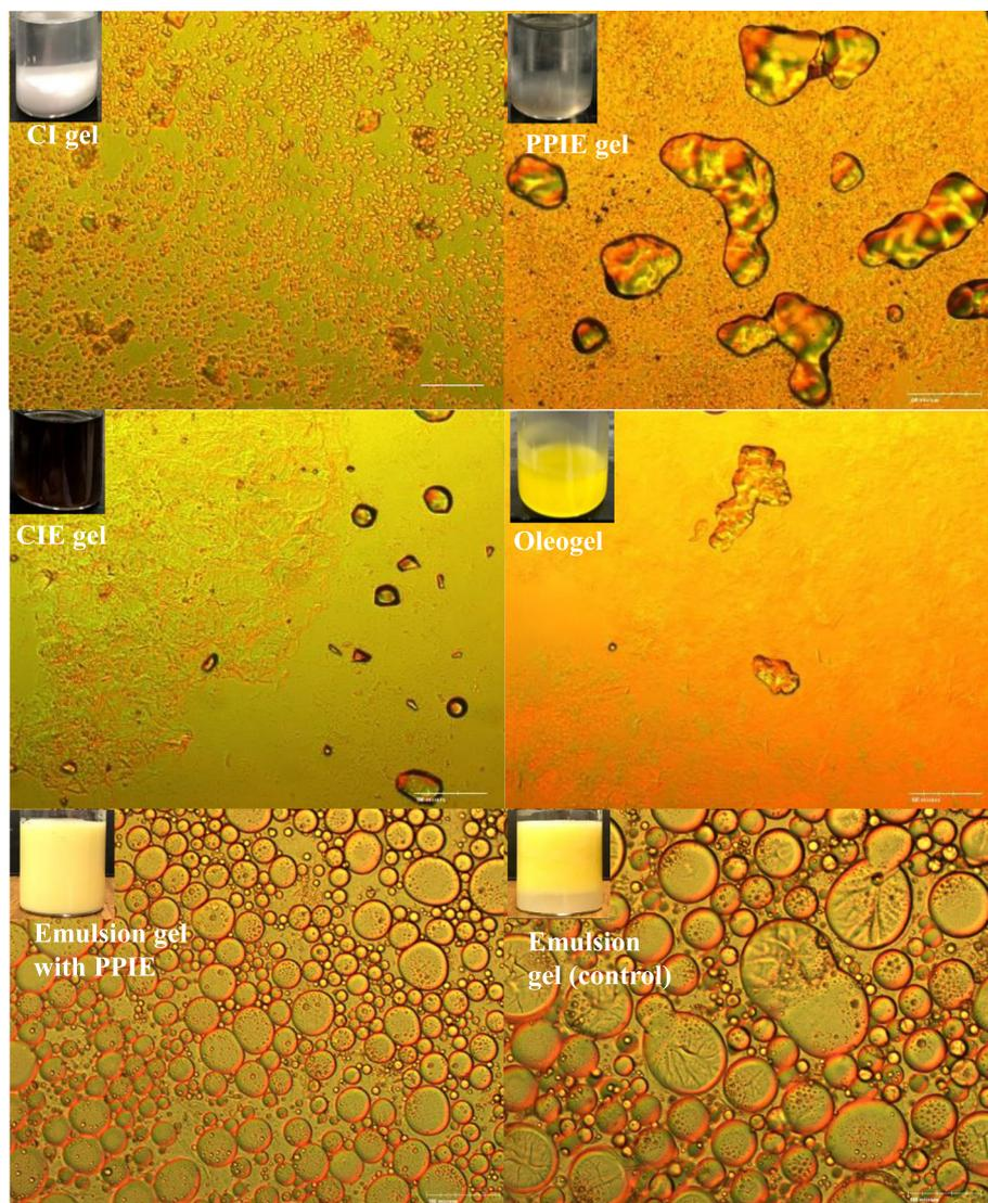
**Fig. 4** Polarized light microscope images of gels and emulsion gels. The first two rows from the top indicate inulin gels and/or oleogel; the third row shows emulsion gel with 1% PPIE and without PPIE (control). CI: commercial inulin from chicory root; PPIE: primary purified inulin extract from JA; CIE: crude inulin extract from JA; MGs: monoglycerides; oleogel is formed by MGs; magnification: 200x; scale bar =100  $\mu$ m
