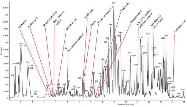
Fig. 2 Chromatogram of the base peak intensity vs. retention time of *tapuy* lees sample. Identified analytes are shown labelled. There are 14 identified analytes from 113 spectral peaks
