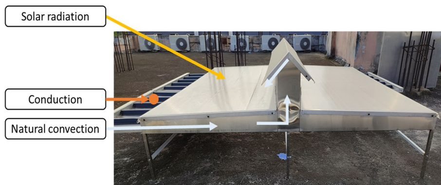
Fig. 1 Various modes of heat transfers take place during the dehydration of onion shreds in the Solar conduction dryer used in this study
